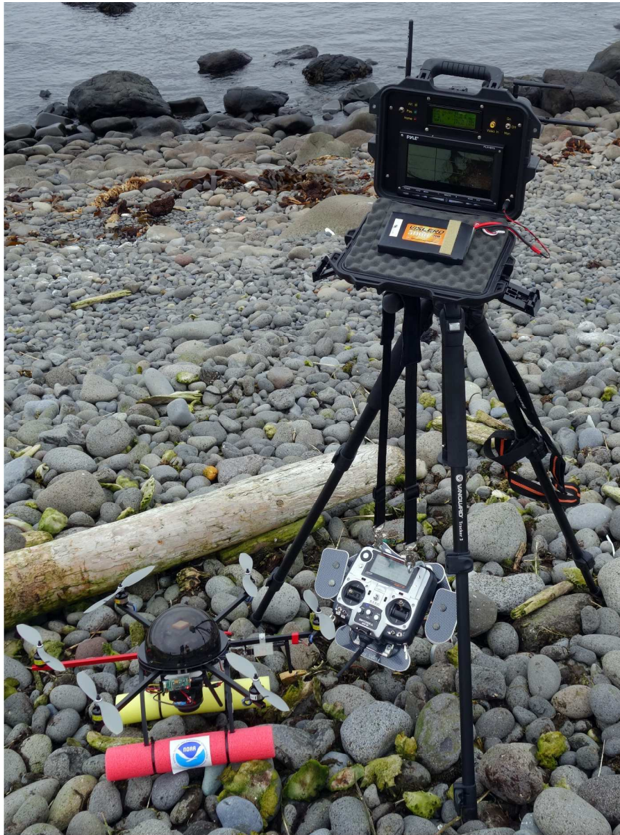
The APH-22 hexacopter system including the 6-rotor aircraft (left), ground station (mounted on the tripod), and the radio control transmitter (bottom, right). 295x397mm (300 x 300 DPI)
