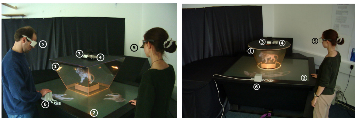
Figure 5.25: The Virtual Showcase prototypes. A Virtual Showcase built from planar sections (left), and a curved Virtual Showcase (right).
