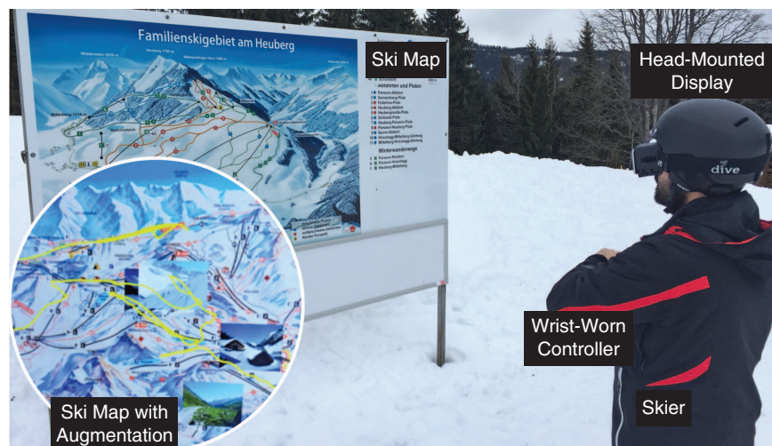
FIGURE 4. A participant browses through digital content overlaid on a panoramic resort map.
