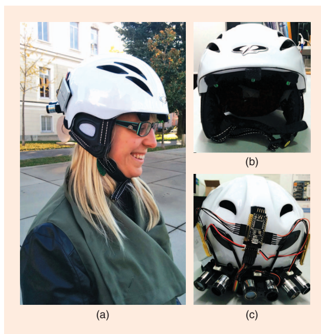
FIGURE 1. (a) A participant wearing an s-Helmet prototype during the off-slope experiment. The (b) front view and (c) rear view of the s-Helmet.
