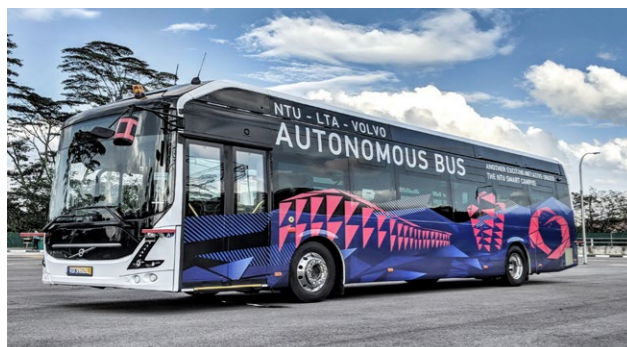
The Nanyang Technological University, Singapore (NTU Singapore) and Volvo Buses are trialling a full size, autonomous electric bus equipped with a comprehensive artificial intelligence system developed by NTU Singapore engineers.
