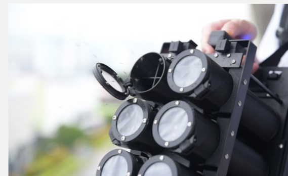
The Mosquito Launcher is a lightweight device that allows field operators to carry more mosquitoes in a single trip, thus reducing the release duration.
