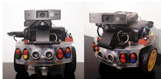
Figure 44: Wheeled robot programmable with BlockWiSARD
