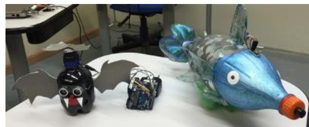
Figure 7: PET bottle Robotic Bat and Robotic Fish
