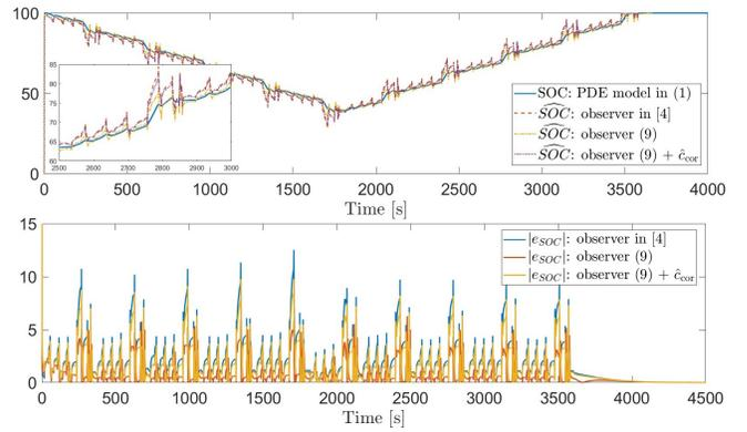
Fig. 3. SOC and  $\widehat{SOC}$  generated by the observer in [4], observer (9) and observer (9) with  $\hat{c}_{cor}$  (top) and norm of the estimation errors  $e_{SOC} := SOC - \widehat{SOC}$  (bottom).
