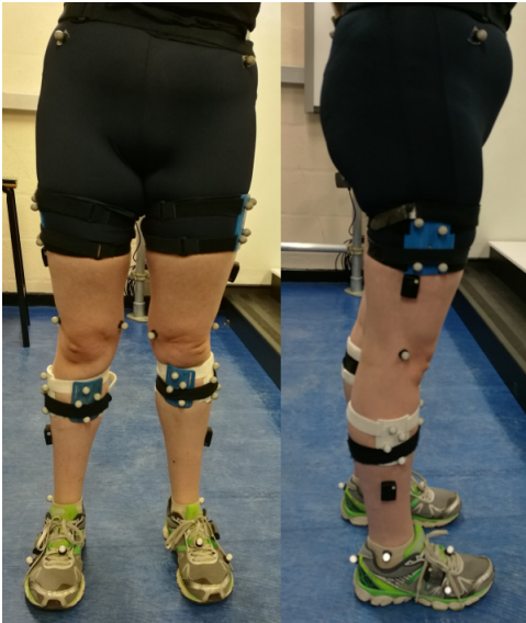
Fig. 3. Placement of inertial measurement units and optical marker clusters on a subject. The Strathclyde functional cluster model was used to analyse gait phases and kinematics. The IMUs were attached to the thigh, shank and foot without restricting their positions.
