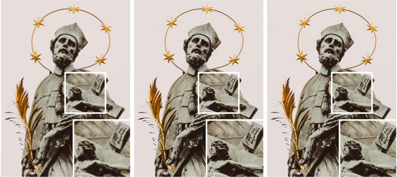
Figure 18. Performance comparison of SISR at scale factor of 4 of bicubic downsampling. The proposed network is RGB based network. Left : input, Center : restoration result, Right : label.
