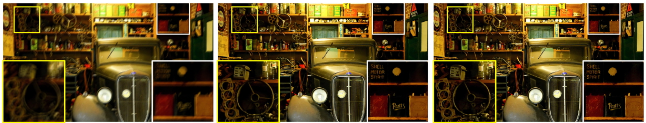
Figure 15. Performance comparison of SISR at scale factor of 4 of unknown downsampling. The proposed network is RGB based network. Left : input, Center : restoration result, Right : label.
