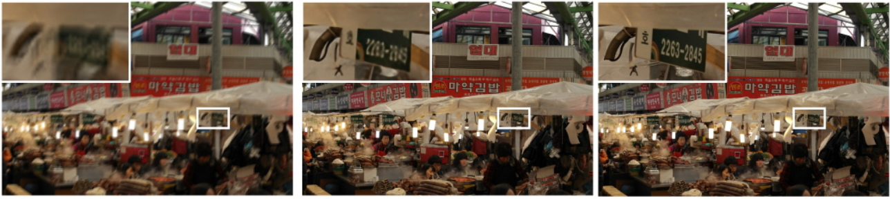
Figure 14. Performance comparison of SISR at scale factor of 4 of unknown downsampling. The proposed network is RGB based network. Left : input, Center : restoration result, Right : label.
