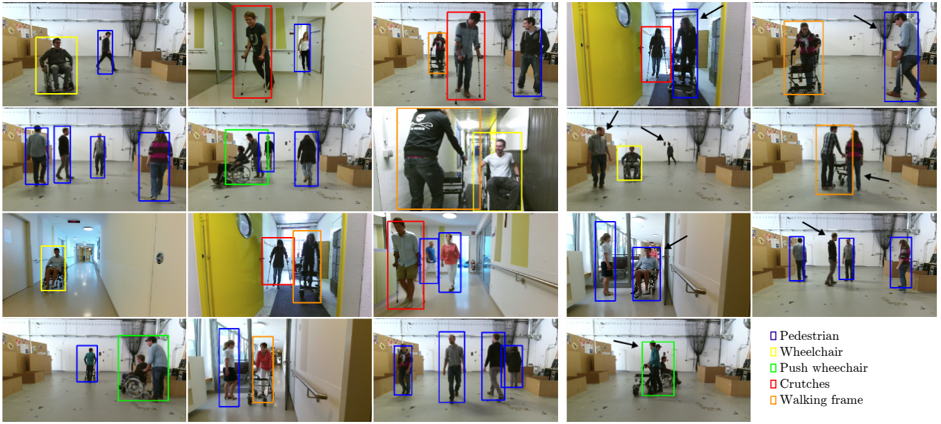
Fig. 6. Qualitative object detection results obtained using our trained Fast R-CNN network. Left: positive examples. Right: cases of failure with missed detections and wrong classifications. We show the RGB image only for demonstration purposes.
