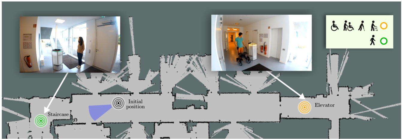
Fig. 8. We use our framework to provide assistance in a person guidance experiment. The robot’s task is to guide all pedestrians to the nearest staircase (left image) and all people with mobility aids to the elevator (right image). We told the test subjects to approach the robot at the initial position and then follow the robot’s predefined speech commands.
