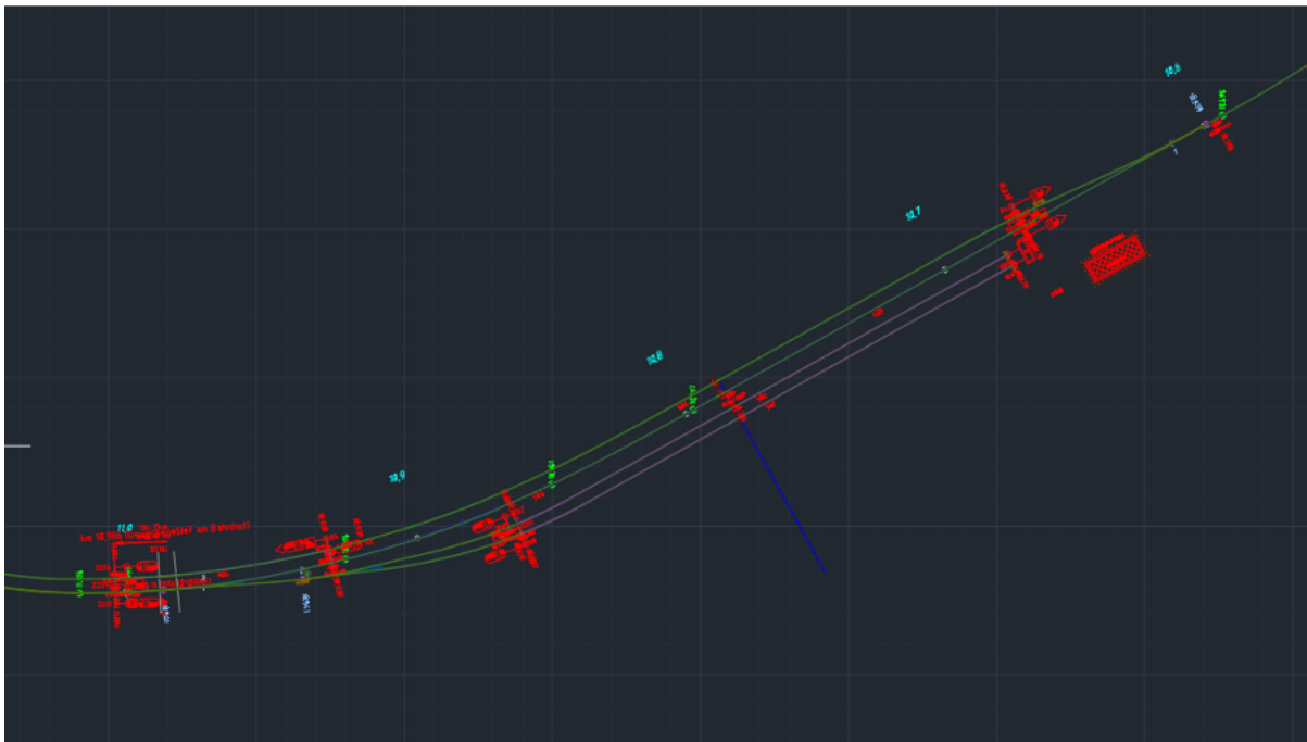
Fig. 2. The railway station Scheibenberg of the Digital Testfield of Deutsche Bahn in ProSig 7.3. The four different tracks together with their signals and endings are visible in the map (best in colors).
