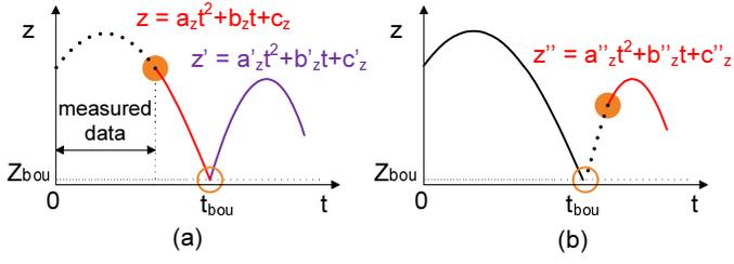
Fig. 4. (a) phase I: rough prediction with bouncing model before ball bouncing; (b) phase II: precise prediction after ball bouncing, the red curve  $z''$  is the predicted ball trajectory after bouncing
