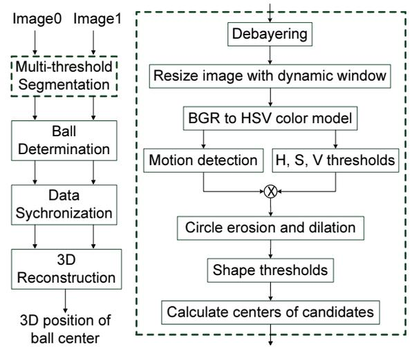
Fig. 2. Diagram of vision processing with multi-threshold segmentation
