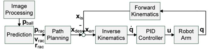
Fig. 5. Control diagram of humanoid 7-DOF robot arm
