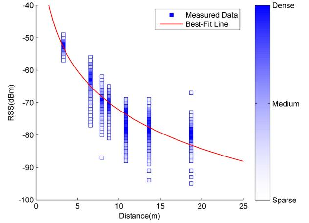
Fig. 4. An example of calibration result for a receiver.
