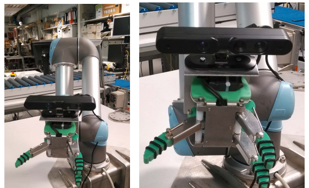
Fig. 19 Experiment setup. A Lacquey under-actuated gripper and an Asus Pro Live sensor are installed at the end of the Universal arm (UR5).
