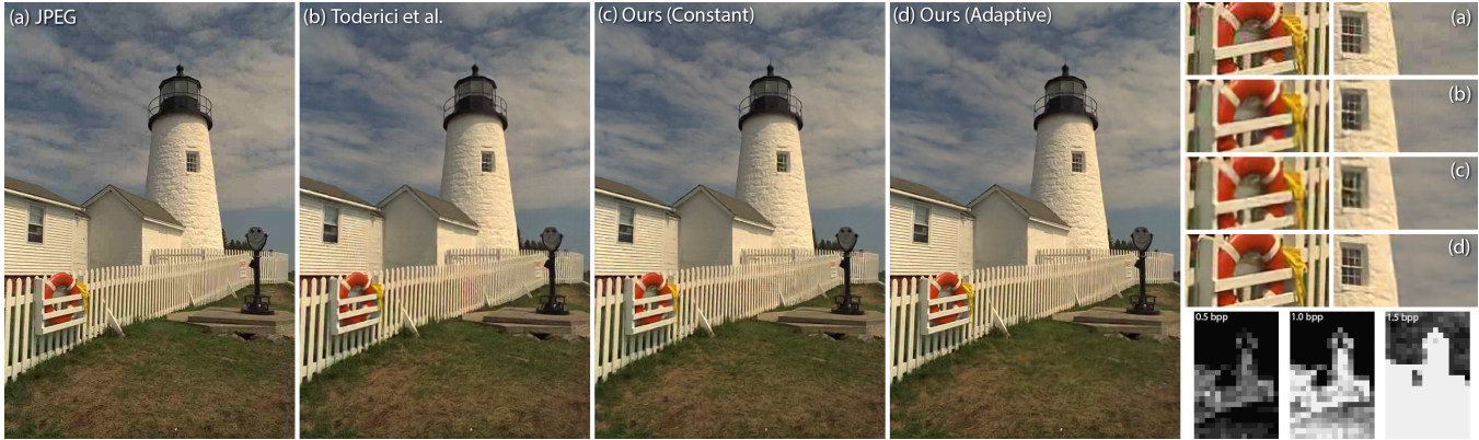
Fig. 6. Reconstructions at 0.5 bpp: (a) JPEG (PSNR=29.552), (b) Toderici et al. [2] (28.270), (c) our method with constant bit rate (28.890), and (d) our adaptive model (30.418). The far right (top) shows two zoomed-in regions for better comparison, while the bottom shows the adaptive bit rate mask calculated at three bit rates.
