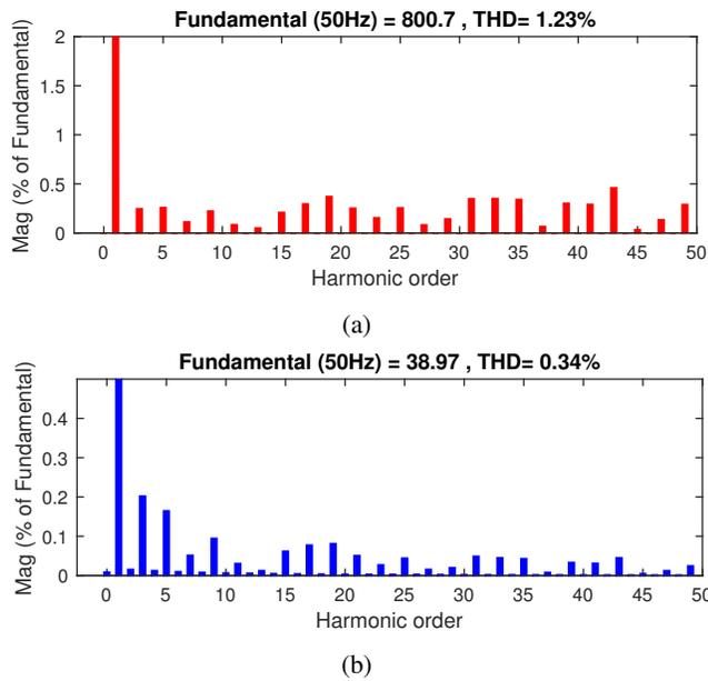
Fig. 6: (a) FFT of the voltage (THD<sub>v</sub> = 1.23%); (b) FFT of the current (THD<sub>i</sub> = 0.34%).
