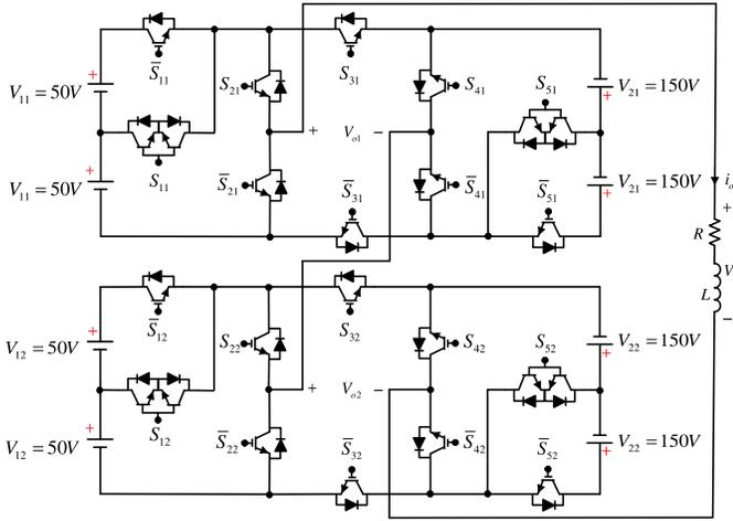
Fig. 4: Proposed 33-level cascaded multilevel inverter power circuit under simulation.
