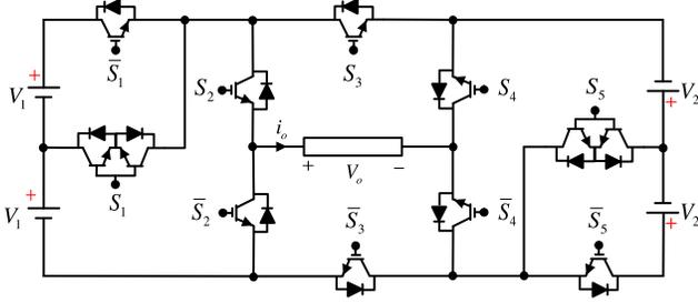
Fig. 1: The proposed 17-level basic inverter.
