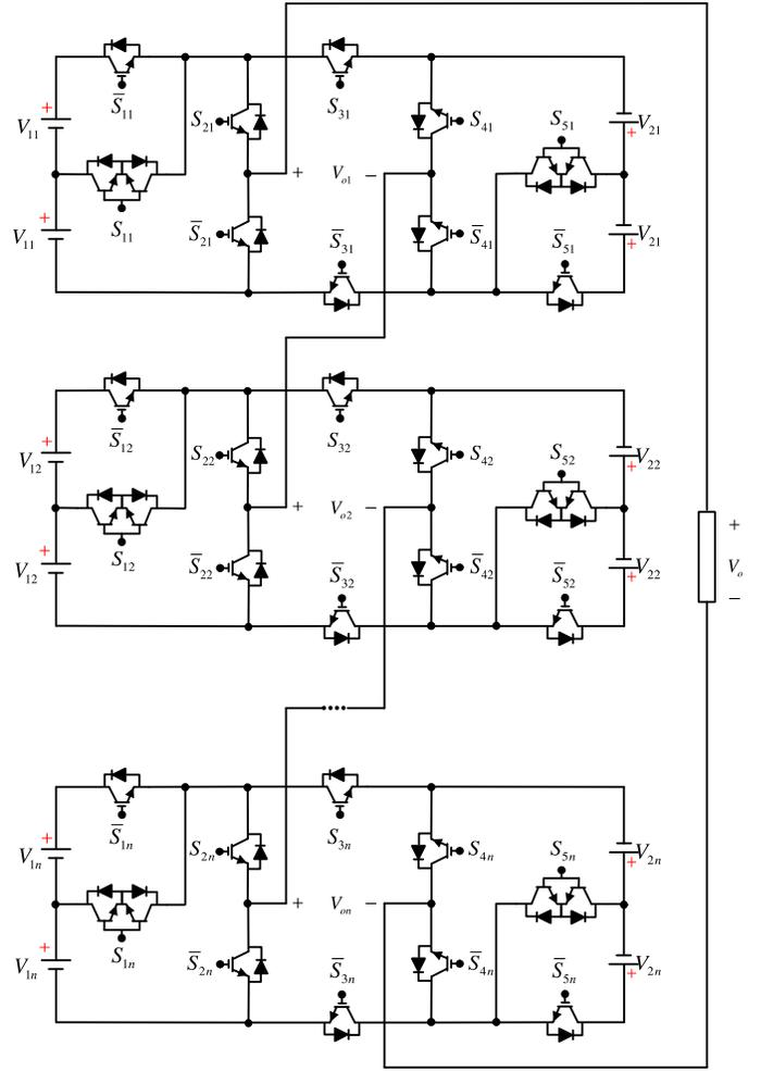
Fig. 2: Cascaded multilevel inverter based on  $n$  number of proposed basic inverter.
