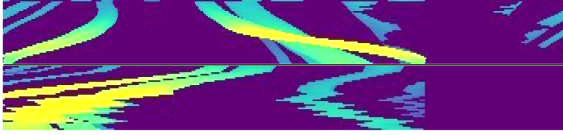
Fig. 3: Visualization of \mathbf{o}_m^t with calibration (top) and without (bottom). When either the robot or a nearby pedestrian moves, the laser scan response will change, so will \mathbf{o}_m^t . We disentangle robot ego motion out to help the policy training.
