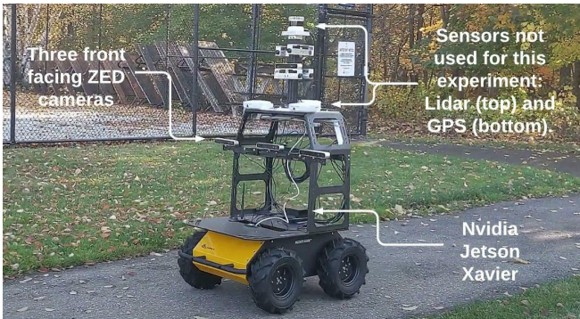
Fig. 8. Clearpath Husky used for ground robot experiments with three front facing cameras mounted in the front.
