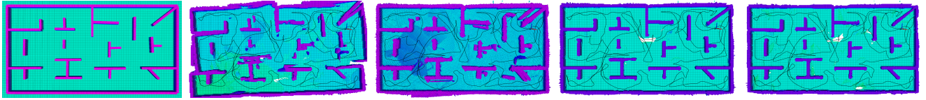
Fig. 6. Mapping result of exploration in simulation environment ( 30 \times 16 \times 3 \text{ m}^3 ) under severe odometry drift (s4). From left to right: the ground truth point cloud, Voxblox, C-blox, our method w/o frame pruning and our method. It can be found that our method can maintain a good global consistency during the exploration flight. If the loop closure result is close to the actual localization, our reconstruction result is approximate to the ground truth.
