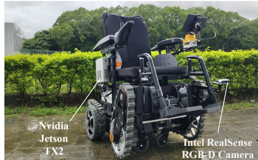
Fig. 1: The robotic wheelchair used in this work. It is equipped with an Intel RealSense RGB-D camera to collect data and an NVIDIA Jetson TX2 to run our S2P2 model.
