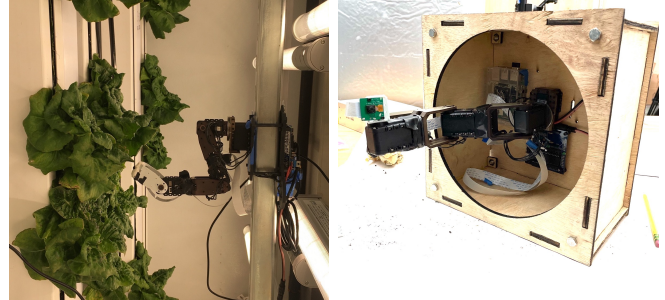
Fig. 3. 4DoF Robot arm with camera used to take a large number of photos from various angles of a single plant. Left: Arm (without wooden cover or CDPR) taking photos of a plant. Right: Arm inside wooden protective cover.
