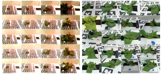
Fig. 9. Left: Example photos from our plant dataset depict the consistency with which our robot is able to photograph different plants from the same relative camera angle. Right: In contrast, photos taken using only the robot arm (Baseline 3) are inconsistent and labor-intensive.
