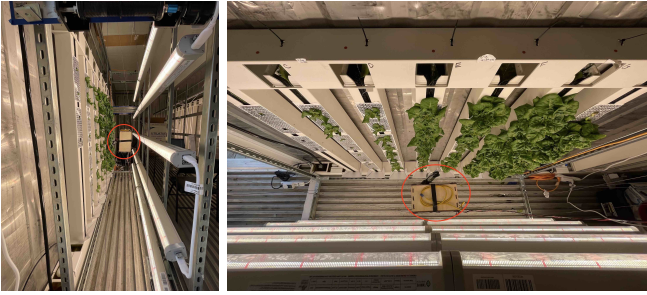
Fig. 1. The robot is placed in a vertical indoor grow chamber between the plants and the grow lights (Left: side view; Right: top view). The robot consists of a CDPR which moves the robot arm (circled in red) from plant to plant to take photos from a wide set of viewpoints.
