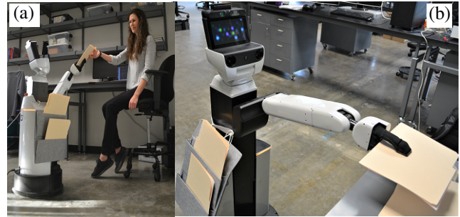
Fig. 1. (a) The Toyota Human Support Robot, which we use as our experimental platform for human-informed work delivery, picking up completed work. (b) The HSR dropping off completed work at the Inventory Station.
