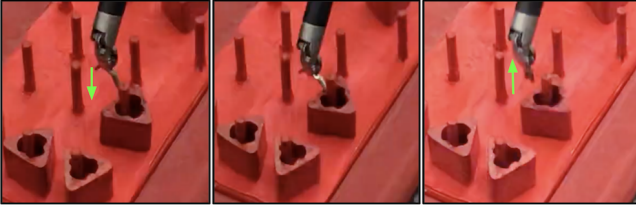
Fig. 3: Time lapse of an example pick failure from the dVRK. The pick operation initially opens the gripper and lowers it (first image), but the gripper only barely touches the block edge (second image). When the gripper closes, it is unable to get the block within its grip as it rises (third image).
