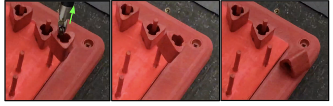
Fig. 5: Time lapse of an example place-fall failure from the dVRK. The placing operation results in the bottom of the block making contact with the top of the peg. When the gripper releases the block and moves up (first images) the block eventually falls off the peg (last two images).
