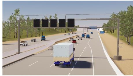
Fig. 6. Real-world evaluation data is collected on a highway (depicted here as digital twin for privacy reasons). Radar and camera sensors are mounted on the gantry above the road, facing into the direction of travel.
