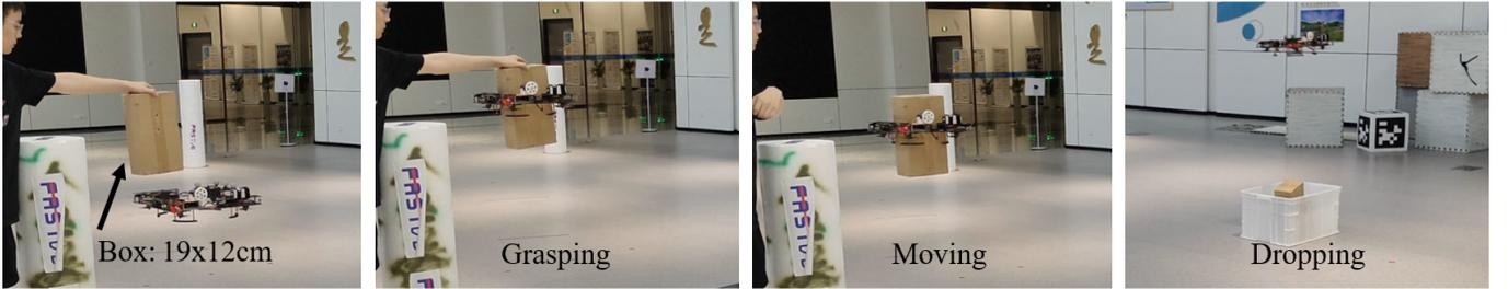
Fig. 10: The vehicle grasps and transports autonomously the target object to the goal position.
