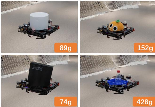
Fig. 12: Ring-Rotor grasps various shapes of objects.
