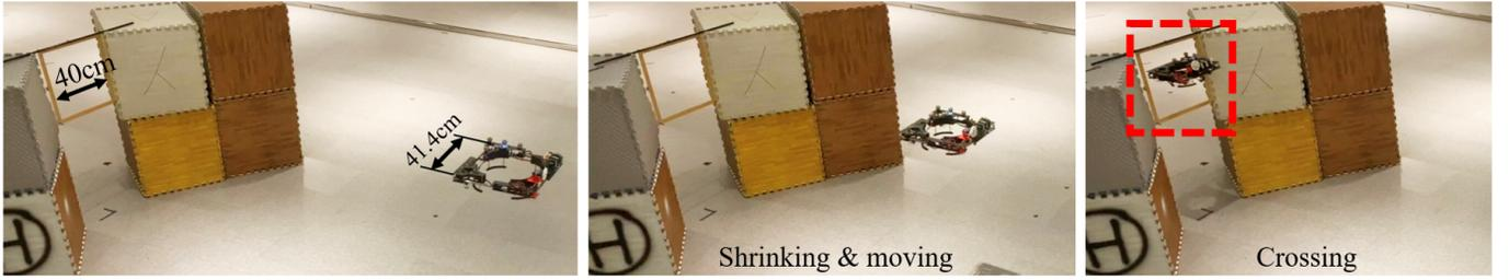
Fig. 8: The vehicle crosses the gap horizontally.
