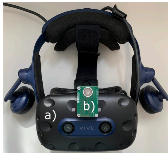
Figure 1: the combined sensor setup comprised of a) an HTC Vive Pro 2 VR headset with embedded optical cameras and b) the \mu RTIS ultrasound sensor featuring a dense microphone array and a broadband ultrasonic emitter.
