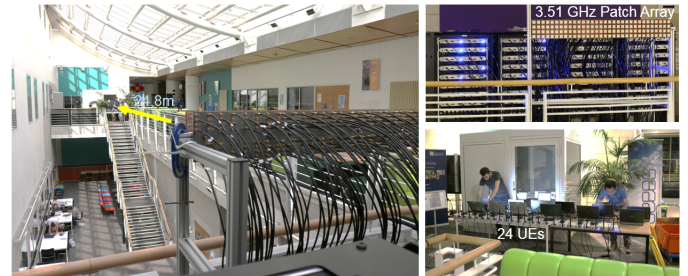
Fig. 9. Second measurement trial with the UEs 24.8m away
