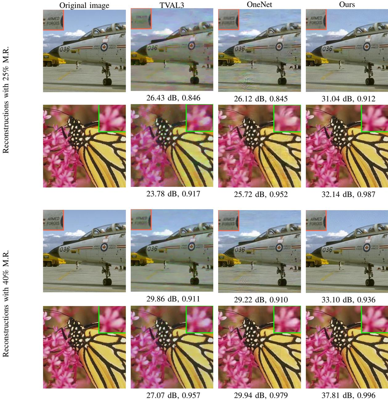
Fig. 11. Qualitative comparisons of images reconstructed from simulated LiSens measurements using TVAL3, OneNet and our approach. Reconstructions from our approach have minimal artifacts and are closer to the original image.
