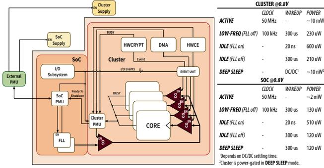
Fig. 2: Fulmine power management architecture and power modes.
