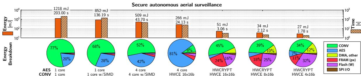
Fig. 8: Secure autonomous aerial surveillance use case based on a *ResNet-20* CNN [10] with AES-128-XTS encryption for all weights and partial results. KEC-CNN-SW and CRY-CNN-SW operating modes at  $V_{DD} = 0.8$  V.
