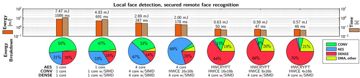
Fig. 9: Local face DETECTION, secured remote recognition use case based on the 12-net and 24-net CNNs from Li et al. [67] on a  $224 \times 224$  input image, with full AES-128-XTS encryption of the image if a potential face is detected. CRY-CNN-SW operating mode at  $V_{DD} = 0.8$  V. We consider that the first stage 12-net classifies 10% of the input image as containing faces, and that the second stage 24-net is applied only to that fraction.
