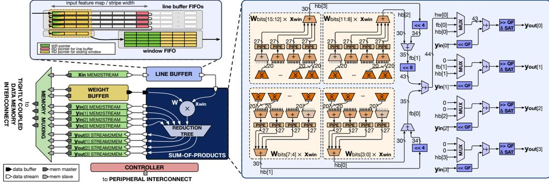
Fig. 4: *Fulmine* HWCE architecture, with the *controller* shaded in red, the *wrapper* in green, and the *datapath* in blue. The diagram also shows details of the line buffer and sum-of-products submodules microarchitecture.
