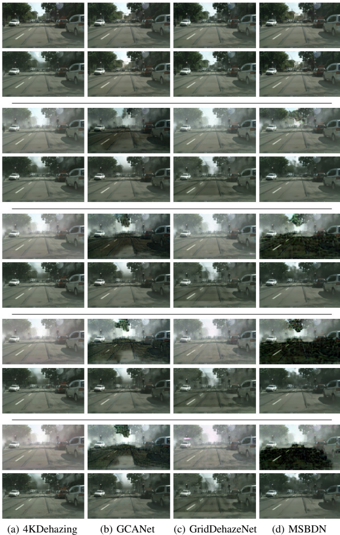
Fig. 10. Image dehazing results obtained by different dehazing algorithms under attack loss L_P^{MSE} before and after defense training. Every two rows of images are in a group. The above images of each group are the results of direct attack (without defense training), and the bottom images are the results of attack after defense training. The \epsilon of two rows from up to down are 0, 2, 4, 6 and 8, respectively. Images are from Foggy-City.
