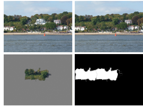
Fig. 3. The image beachwood (upper left) is forged with a green patch (bottom left) to conceal a building (upper right). A ground truth map (bottom right) is generated where copy-moved pixels are white, unaltered pixels are black and boundary pixels are gray.
