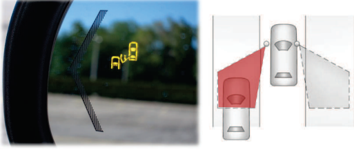
Fig. 1. General Motors' SBZA system on a 2011 Cadillac Escalade [35]
