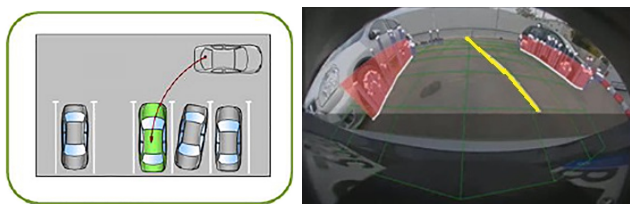
Fig. 5: Parking with cameras can be guided by road markings and not just objects, unlike Ultrasonic and Radar.
