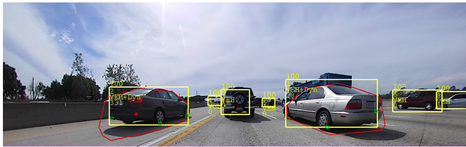
Fig. 18: Reorganization combines Reconstruction’s dynamic object detection output (red polygon) and Recognition’s object detection (yellow box).
