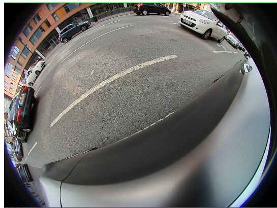
Fig. 8: Significant deviation from translation invariance is evident in fisheye cameras.
