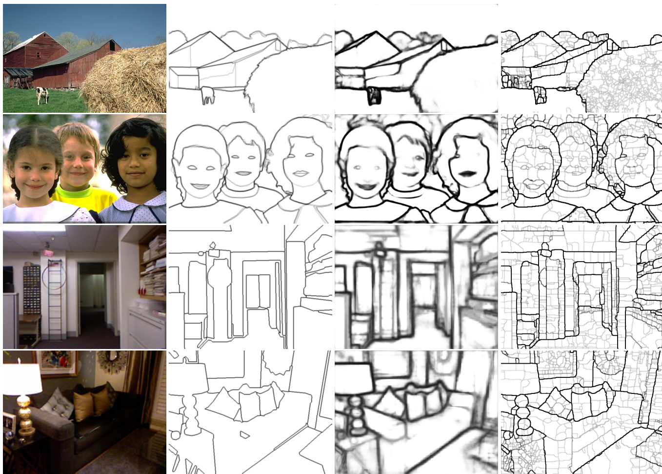
Fig. 6: Some examples of RCF. Top two rows: BSDS500 [9]. Bottom two rows: NYUD [30]. From Left to Right: origin image, ground truth, RCF edge map, RCF UCM map.
