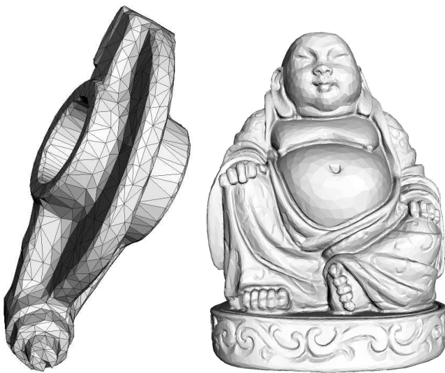
Fig. 12. Coarsened versions of the rockerarm model (1000 vertices) and the buddha model (20k vertices).
