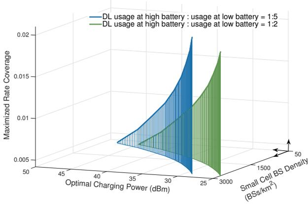
Fig. 4. Maximized rate coverage and optimal charging power with respect to the  $\lambda_2$  and DL usage ratio  $\frac{u_h}{u_\ell}$  ( $\lambda_1=10$  BSs/km<sup>2</sup>,  $\lambda_u=1 \times 10^4$  users/km<sup>2</sup>,  $P_1=43$  dBm,  $P_2=23$  dBm,  $W=10$  MHz,  $\theta=1$  Mbps,  $\alpha=4$ ,  $\beta=5$ ,  $\hat{r}_a=2$  m,  $G_m=10$  dBi,  $G_s=-7.4$  dBi [20]).
