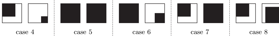
FIG. 4.1. Illustration of the sparsity patterns of the reduced Hessians \nabla_{\mathcal{L}_f^c}^2 g(x) and \nabla_{\mathcal{L}_f^c}^2 h(x) for the cases 4–8 in Tab. 4.1 and Lem. 4.7. White areas correspond to zero blocks in the Hessians, black areas to non-trivial blocks. The black areas in case 4 correspond to the non-trivial submatrices \nabla_{\mathcal{L}_g^c}^2 g(x) and \nabla_{\mathcal{L}_h^c}^2 h(x) on the l.h.s. of Eq. (4.11).
