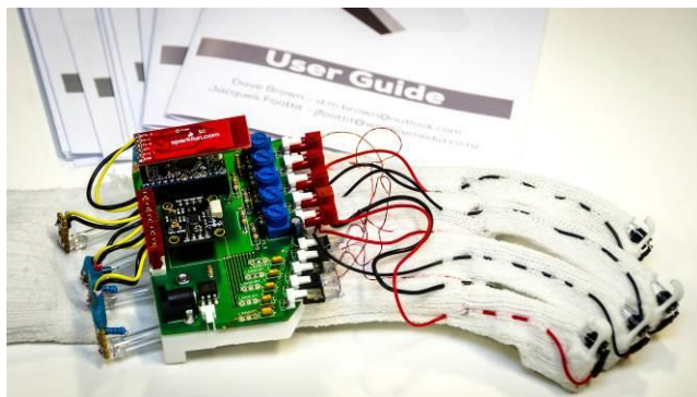
Figure 2. The final haptic glove.
