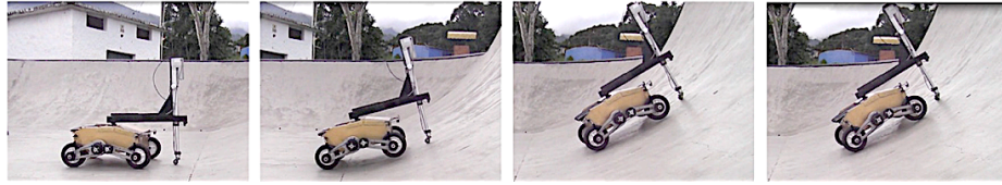
Fig. 5. First test: Image sequence of Lazaro moving upwards on a half-pipe with \alpha \approx 0^\circ .
