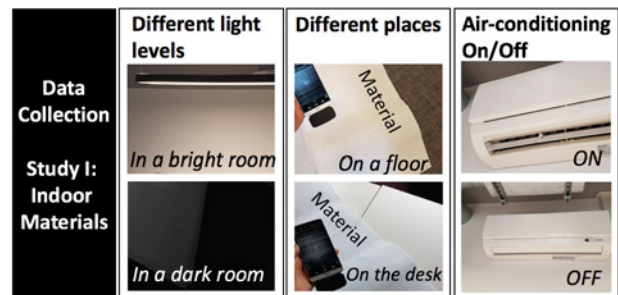
Figure 5. Data collection for Study I: thermal images of indoor materials were recorded under different conditions (lighting, place, air-conditioning, direction and distance).
