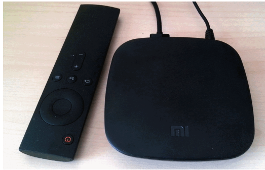
Fig. 1. The Xiaomi MiBox, a TV Set-top box (STB) with a simple remote can turn any TV with an HDMI socket into a Smart TV with the Android TV OS. (Source: Wikipedia, CC BY-SA 3.0 license)
