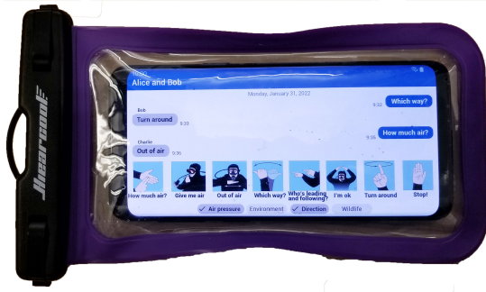
Figure 2: User interface of our messaging system on a phone within a water-proof case.
