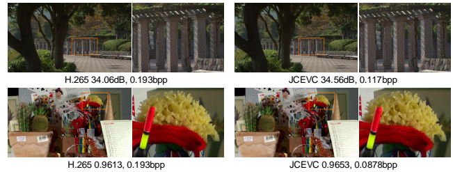
Figure 1: Reconstructed frames with the H.265 (x265 LDP very fast) and our JCEVC. The JCEVC reduces the bit-per-pixel (bpp) of H.265 by almost half whilst retaining competitive PSNR or MS-SSIM. In the view of video coding, the JCEVC achieves a significantly higher RD performance.
