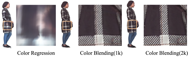
Fig. 14. Results of different ablation settings for texture prediction. From left to right, they are the results of color field estimation, and our blending weight field estimation with 1K and 2K images, respectively.
