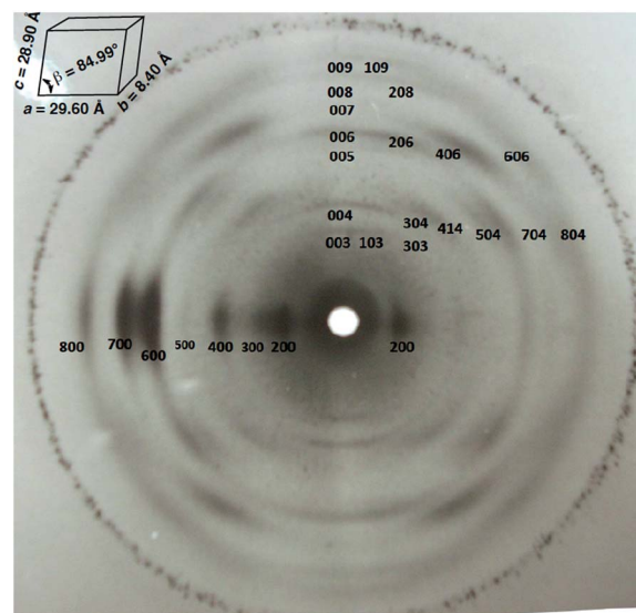
Fig. 1 X-ray diffraction image of H 4 TPPS 4 J-aggregates and inferred unit cell dimensions (space group P2 1 with four porphyrins in the unit cell); h , k , l parameters for strong, medium, weak and broad spots are shown. The outside ring is the distance control (powder silicon standard, 3.1355 Å). For the comparison of experimental vs. calculated distances see table in the ESI. †
