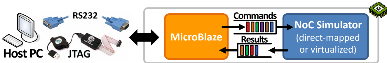
Figure 1. High-level block diagram of platform consisting of Host PC connected to a Xilinx ML605 Development Board.
