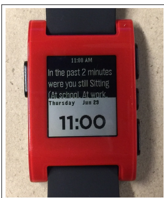
Figure 3: Watch — confirmation notification. The same notification from the phone scrolls on the top half of the watch app. If the user’s context remained the same, they can reply “correct” by pressing the top-right button.
