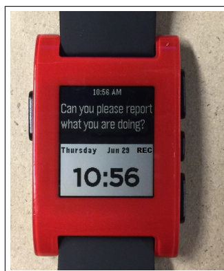
Figure 4: Watch — open-ended notification. This is only useful as a reminder; to initiate reporting labels the user has to go to the phone. During a 20-second recording window, the text “REC” is shown in the bottom half.
