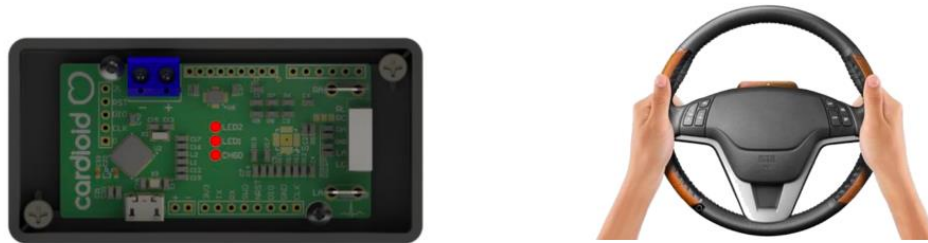
Figure 3-75 CardioWheel embedded system and steering wheel cover.
