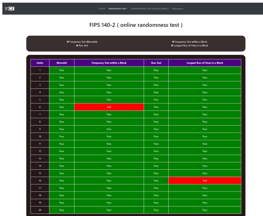
Figure 3-66 Randomness test's P-value results according to FIPS 140-2
