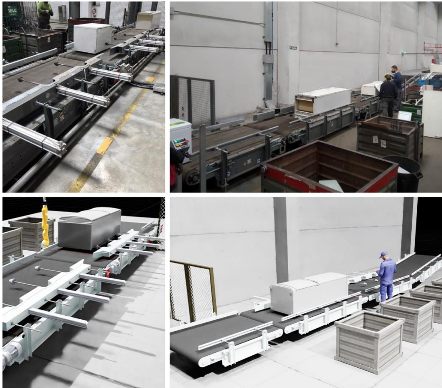
Figure 3-29 Actual disassembly plant (top) and simulated scenario (bottom).
