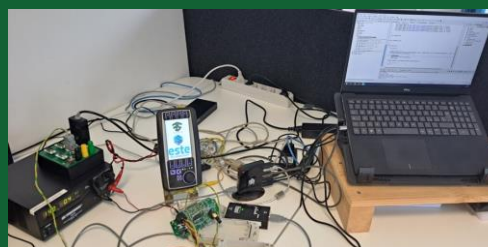
Test-bench based on Arm Unity
