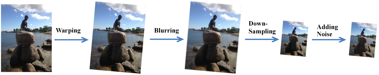
Fig. 3 The imaging model employed in most SR algorithms.
