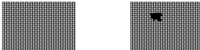
Structure without Defect and Defect hole
